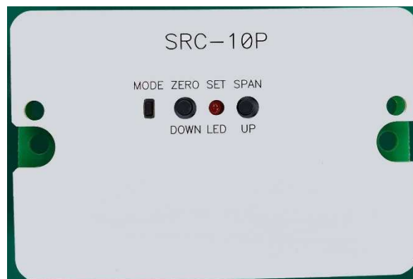
Fig-19. Adjustment of current transmitter
